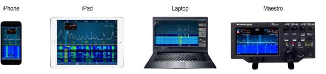
With SmartLink and a FLEX-6600/FLEX-6600M you can operate your radio from almost anywhere! Just take an iPhone, iPad, Laptop or Maestro with you and instantly connect to your radio with virtually no setup required.
